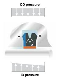
If the sleeve were rigid, the pressure would drop almost linearly along this route, and leakage would be high. Instead the pressure distributions on the outside and inside of the seal produce a turning moment (M) that tilts the seal to bring the 'atmosphere' edge of the seal sleeve into close proximity to the shaft, stemming the leakage.
